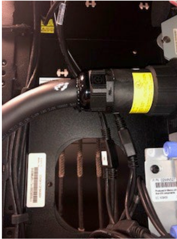
Figure 3: Bottom Exiting Line Cord
