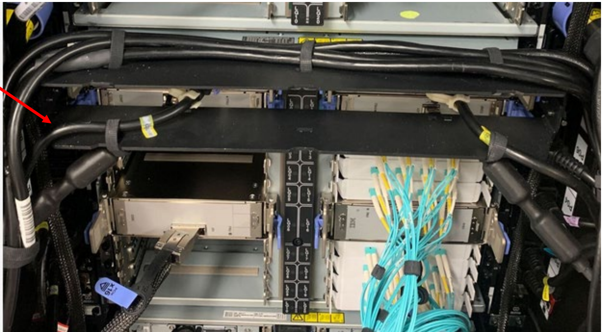
Figure 19: Cable Management Bracket
