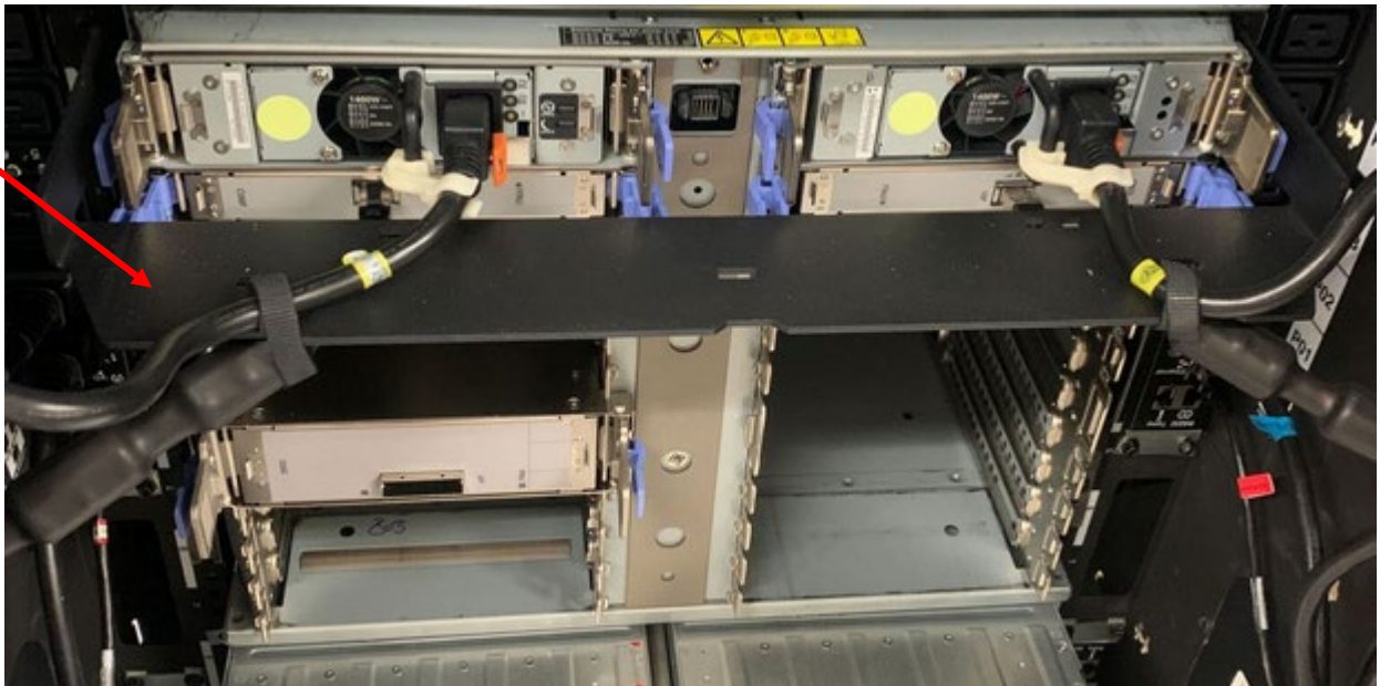
Figure 18: PCIe Drawer Cable Management Bracket
