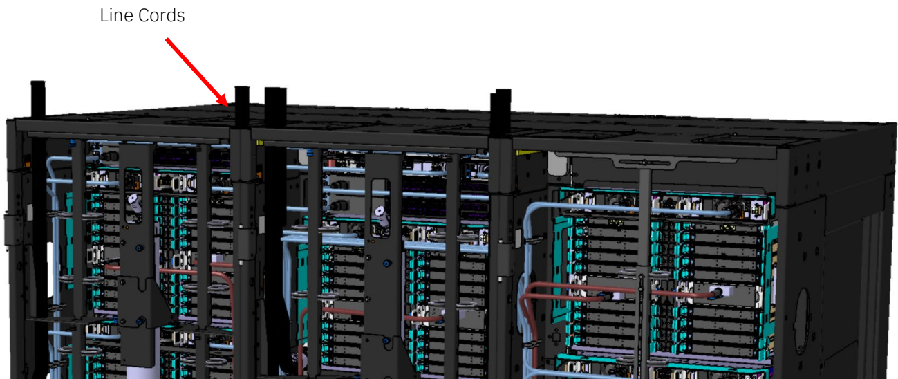
Figure 4: Top Exiting Line Cords without an Enclosure (FC 7816)
