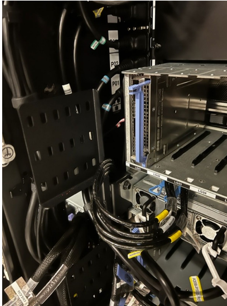
. Figure 48: Neatly Routed SMP cable
